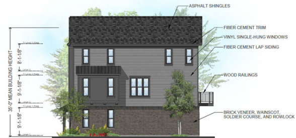
Typical Side Elevation Scale: 3/16" = 1'-0"
