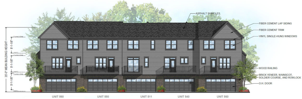
Typical Rear Elevation Scale: 3/16" = 1'-0"
