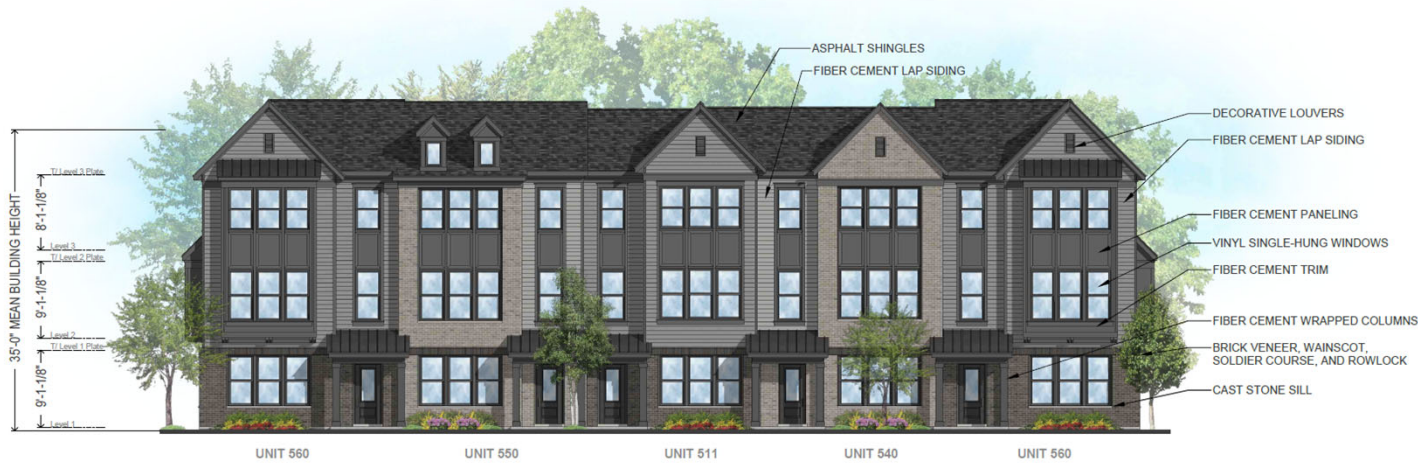
Typical Front Elevation Scale: 3/16" = 1'-0"
