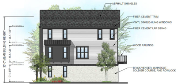
Typical Side Elevation Scale: 3/16" = 1'-0"
